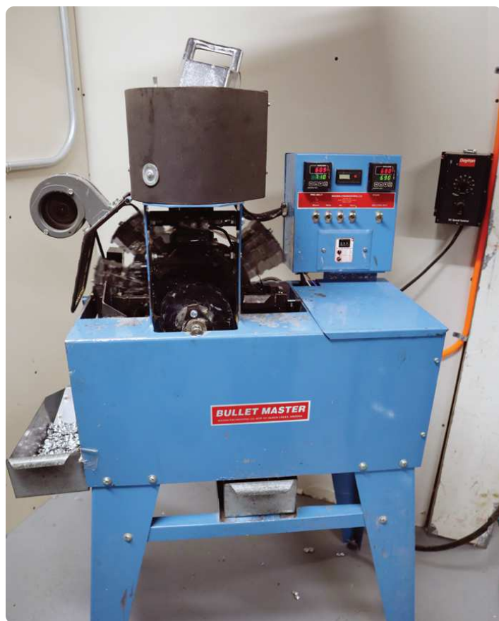
Above —Polymer coated bullets air dry before heat treat. Below —The Bullet Master MK6 at work, note lead in pot.
