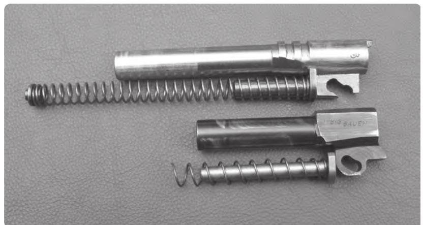
Below —The Browning style linkless barrel from a Star Super SM (top) compared to a SIG P238 barrel.
