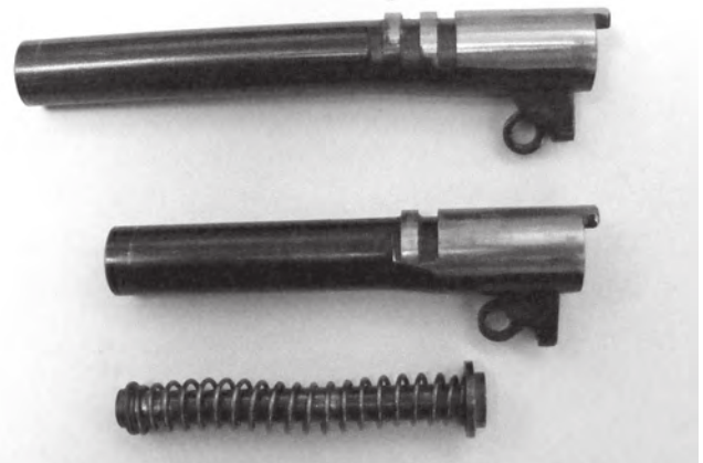
Above —The linked barrels of an S, top, and a DK, bottom—conventional Browning short recoil system.
