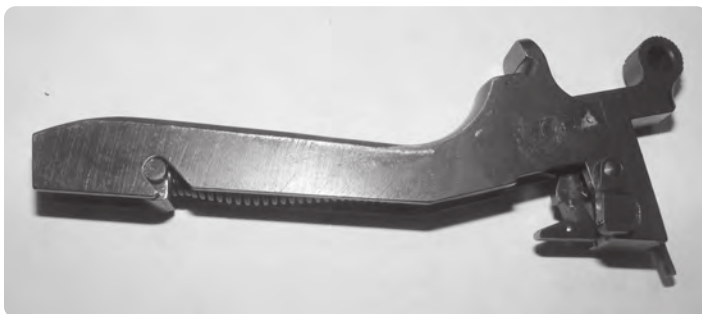
Star 28/30/31—Mainspring, sear, disconnecter, hammer—all in one removable unit without driving pins.
