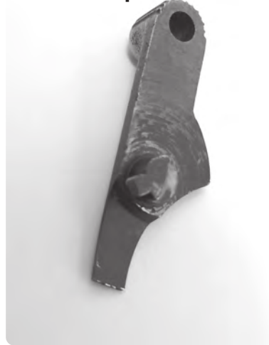
The safety lever with the tip broken off.
