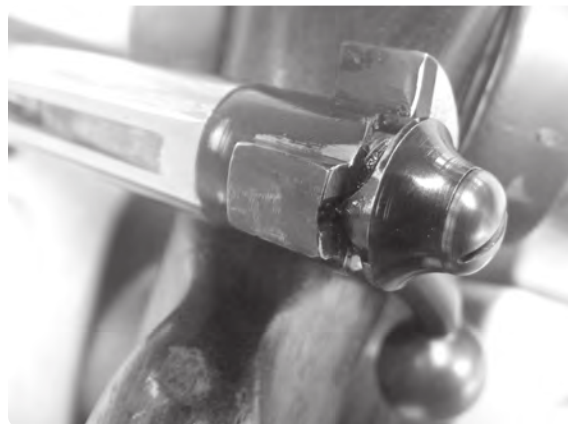
Below —The left lug is massive for a .22, the bolt handle root is the other lug.
