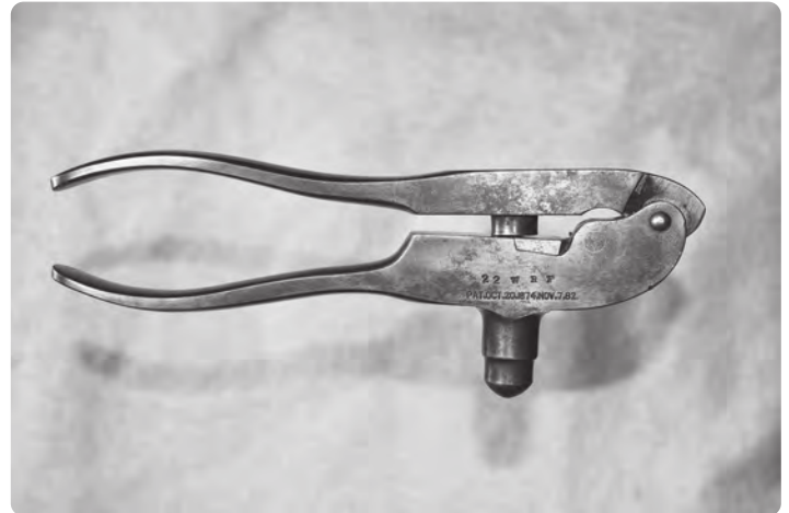
Plate 9, left below —the Hole through the Extractor plate into the seating chamber. Plate 10, right below —Primer seating stud ground flush with tool.
