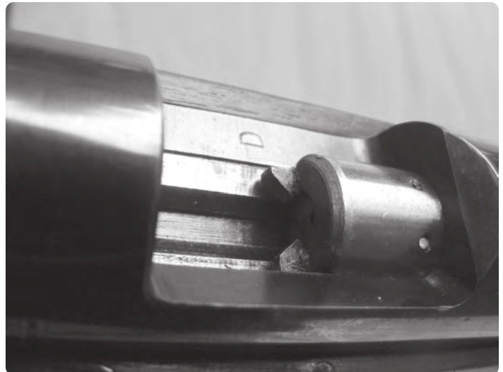
Above —Note the solid receiver with a trough for the cartridge. Also the "D" stamped into the Receiver.
