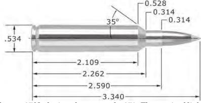
**27 Nosler.** Nosler admits that the new 27 Nosler is an homage to the 270. The case itself is based upon the 404 Jeffrey. Maybe you want 400 FPS more than can be wrung out of a .270? The 27 will do that. Expect 11 inches less drop than the .270 at 500 yards. Twist rate of barrels chambered in Nosler's latest cartridge is 1:8.5-inches for outstanding stability at longer distances. One bullet is the Trophy Grade 150 Grain AccuBond spitzer but I see that other bullets are available.
