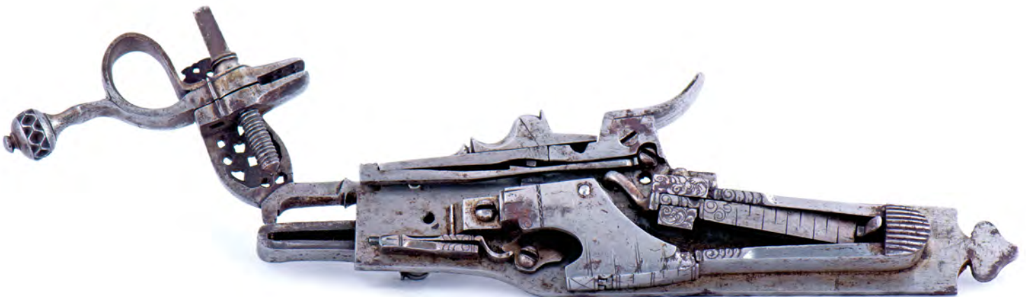
Below —The interior view reveals the workings. At right end of this photo is the heavy mainspring that powers the wheel. The pan is at the top—look for the black hole under the pan cover. Even the springs merit some decorative engraving.
