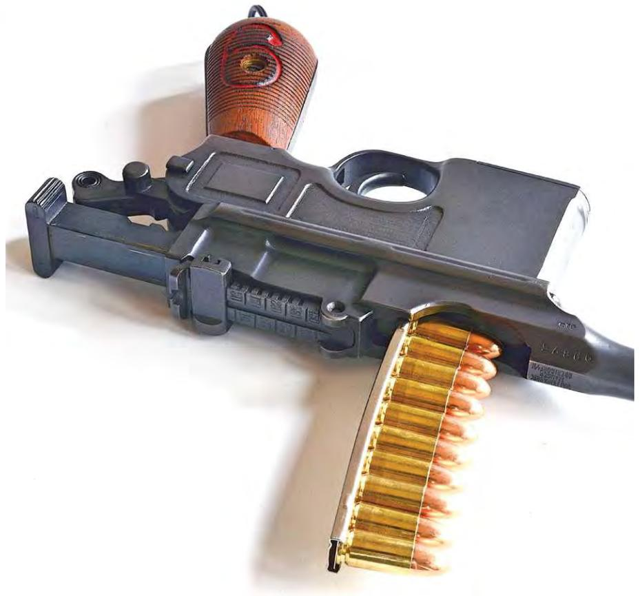
**Right**—Another view of the C96 with bolt to the rear, stripper clip inserted, ready to load.
