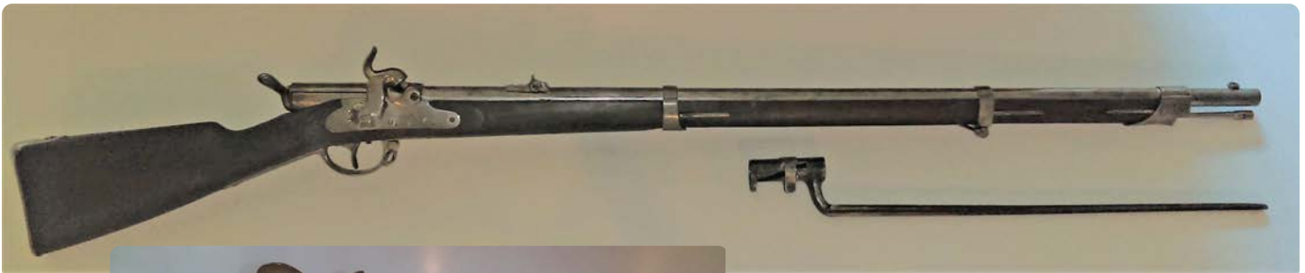
Above—The Bavarian M1858/67 Podewils-Lindner, a stopgap breech-loading conversion. At left—Inset shows breech open and hammer cocked.
