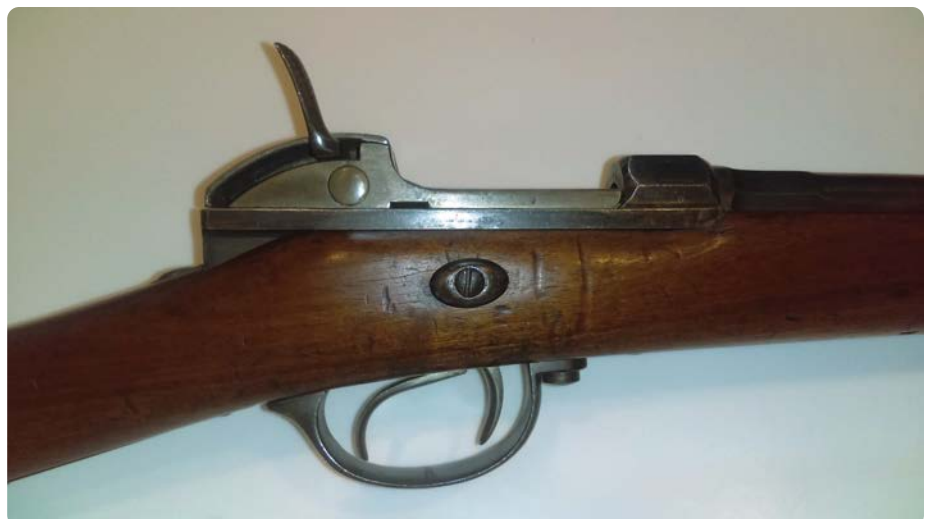
Right—The Werder breech, showing the cocking handle in its curved slot. The trigger guard contains both the trigger (rear lever) and the breech block release (forward lever).
