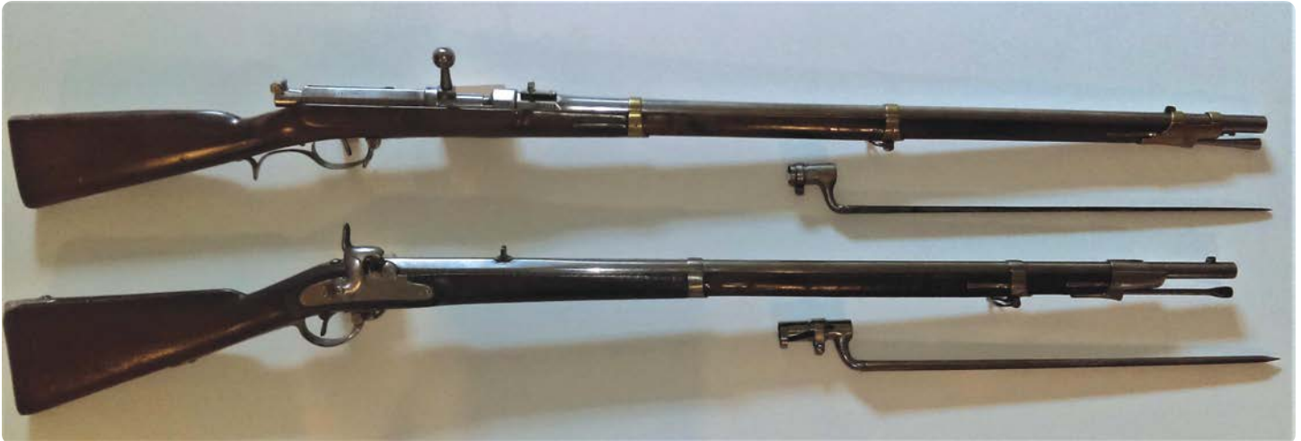
Above— Prussian M1841 Dreyse (top) vs. Austrian M1854 Lorenz (bottom, similar to the Bavarian M1858 Podewils). A very uneven match-up, as the Bavarians found out in 1866.
