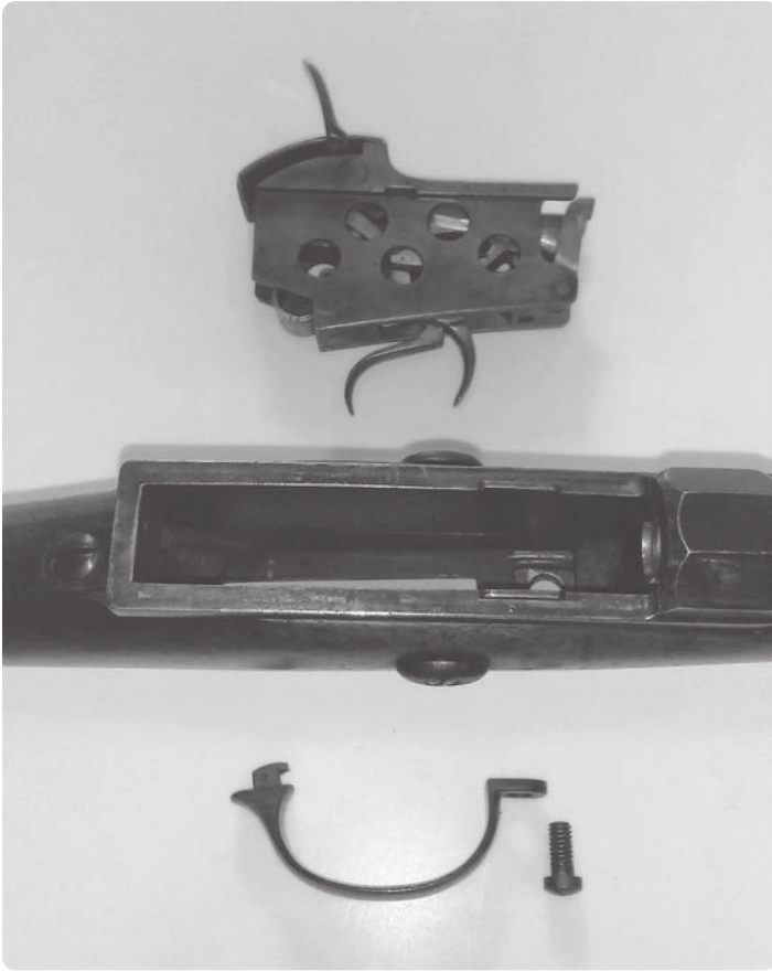
Above left—Werder disassembly: Removing one screw in the trigger guard allows the lockwork to be removed from the receiver.
