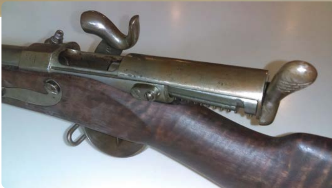
Above—The Bavarian M1858/67 Podewils-Lindner, a stopgap breech-loading conversion. At left—Inset shows breech open and hammer cocked.
