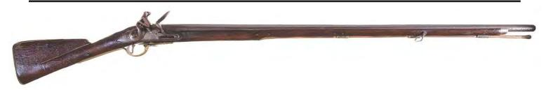
**Above**–This photo is of an original Brown Bess musket. The caliber is .75"–smoothbore and designed for rapid reloading, not accuracy. Basically the same firearm was used by the British for 30 years.
